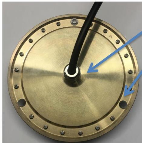
Apply Sealant around this edge and around the cable gland
